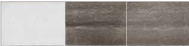
Bitumen roofing membrane with a smooth, reflecting acrylic coating on top
