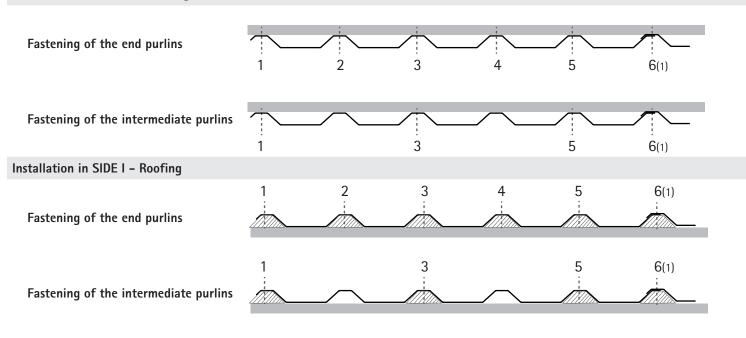
It is recommended to use a light coloured flexible butyl seal between 2 sheets to ensure a good waterproofness.
