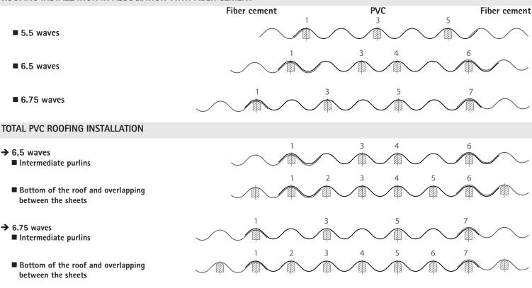
It is recommended to use a light coloured flexible butyl seal between 2 sheets to ensure a good waterproofness.
