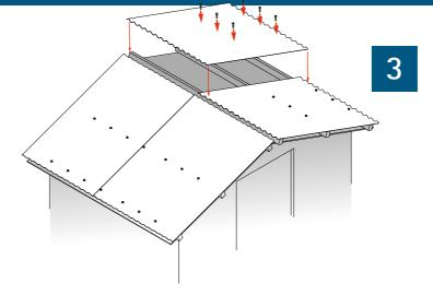
Place and fix the roofing sheets by fixing them to their supports without putting the fixings on the outer ends. These should be positioned at the same time as the ridge cap / corner flashing cap or front plate fixings.
