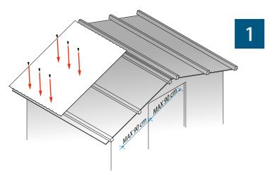
The first fixings are to be put at the top of the waves No. 5, 8 and 11. The wave on the edge (the one on the side) will be fixed when the lateral front plates are installed.
