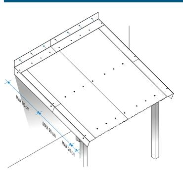
The fixing distribution and installation procedures are the same, whether for a roof or a canopy.
