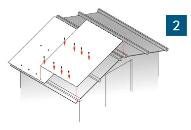
Place the second sheet so that it overlaps 2 waves of the first fixed sheet.
