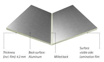
Processing the high-quality cladding panel is extremely simple: mill a small groove into the back of the panel and you can bend RENOLIT BENDIT to the exact angle you need. Any angle up to 90 degrees is possible. The fold is positioned exactly where you want it, and the beautiful surface can withstand it all.
