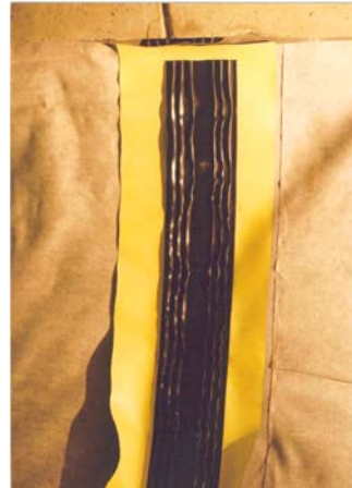
Geomembranes with welded water stops produced in prefabrication
