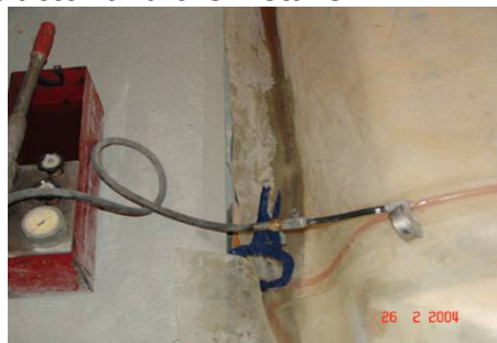
Control by coloured liquid
